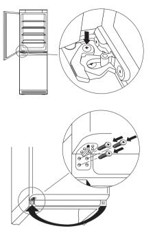
Place the lower door bearing with the bearing pivot in the lower left of the freezer compartment door and fasten.
